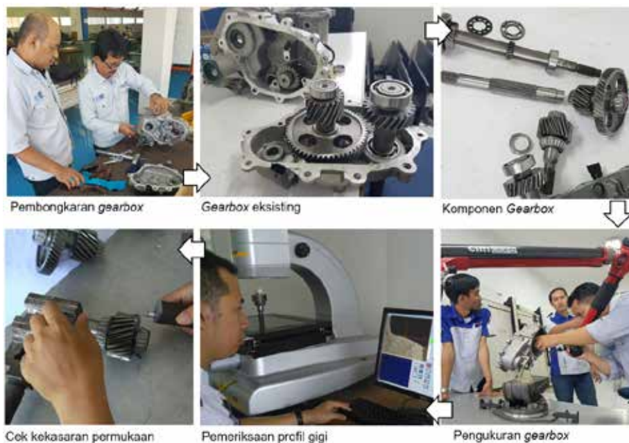
Gambar 5. Proses rekayasa balik sistem transmisi gearbox
